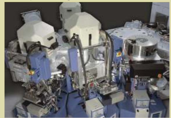
A Compacta with ESA allows to open the cover of a vacuum chamber in different angles.
