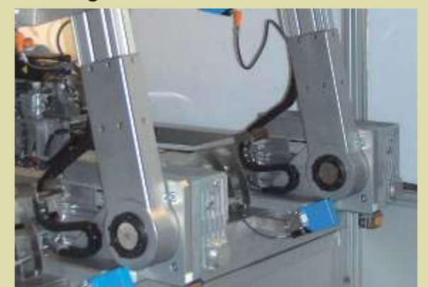
The angles of the pivot arm can be adjusted in different pre-defined positions with ESA.
