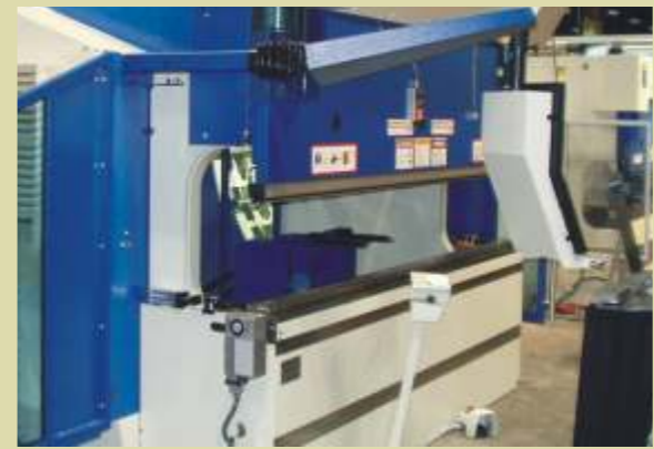
The Compacta precisely adjusts the crowning die unit of press brakes. With the ESA it is possible to pre-define recurring adjustments.
